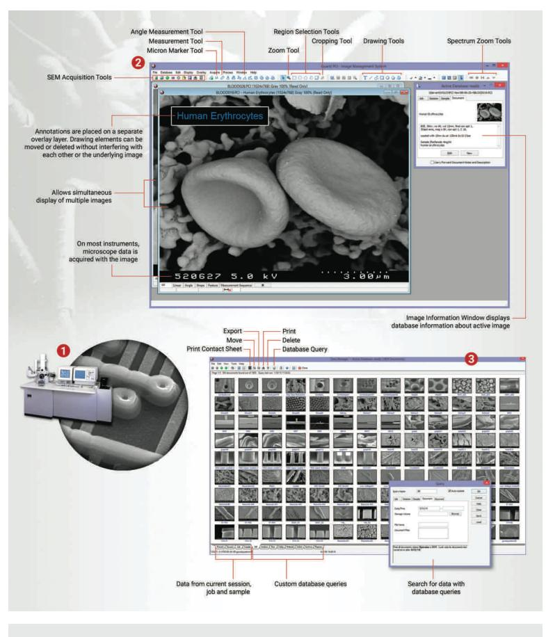
PCI acquires high-resolution, slowscan images from any SEM or STEM. A complete suite of image processing, annotation and analysis tools is included.
